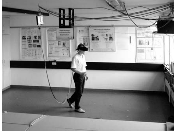
Figure 6. User environment for MC experiments. The user wears a head mounted display. Head motion is tracked by a magnetic tracking system.
