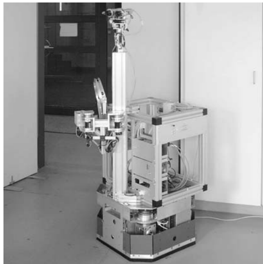
Figure 9. Wheel-based mobile teleoperator with stereo camera unit.
