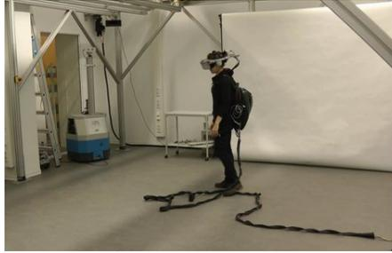
**Fig. 1.** User in the telepresence System, wearing HMD and backpack computer for processing.
