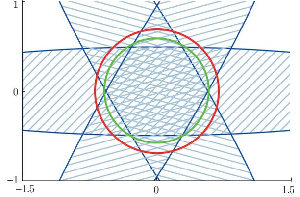
Figure 4. The illustration of the slightly adapted Example 1 from [15]. The covariances  $\mathbf{P}_1, \mathbf{P}_2$ , and  $\mathbf{P}_3$  are depicted in blue, the bound obtained by the natural CI generalization for more than two estimates in red, and the (optimal) tight bound in green.
