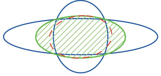
Figure 3. The ellipse of a bound of the fused estimate in green. The ellipses for specific cross-covariance matrices, e.g., the one in dashed red, are enclosed by the ellipse of the bound.
