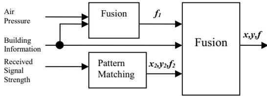
Fig.1. Fusion structure.  $f_i$  is the floor estimation by fusing barometric sensor with building information.  $(x_2, y_2, f_2)$  is the 2-D coordinate and the floor index estimated using the WLAN signal.  $(x, y, f)$  is the final estimated 3-D location.
