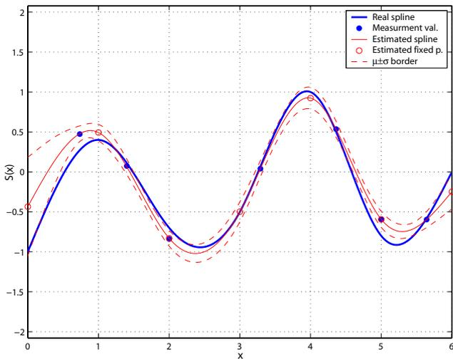
Fig. 4. Single Spline with 7 control points. The first graph shows the starting values, the middle one is after three measurements and last one is after seven measurements. The thick blue line is the real spline, the red thin one is the estimated spline and the red dashed lines are the  $\hat{x}_p \pm \sigma_p^2$  borders. The blue filled dots are measurements, the red ones are the estimated control points. The units on the axes are arbitrary.
