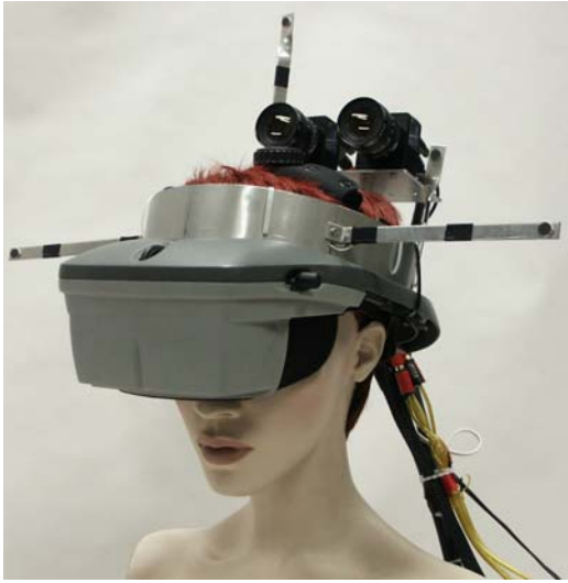
Figure 4: Experimental AR System with audio tracking.
