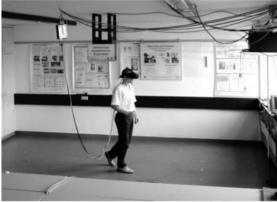
**Figure 8:** *User environment used in the experiments. Available floor space is about 4 m by 4 m. The user wears a HMD and head motion is tracked by a extended range magnetic tracker.*
