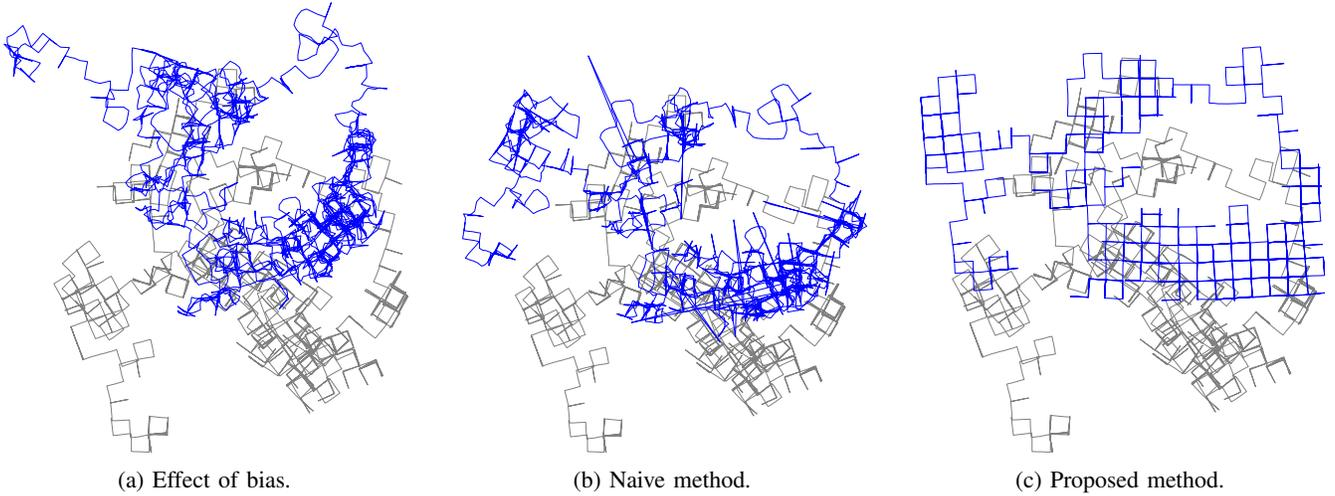
Fig. 2: Different solutions for the Manhattan3500 data set. Loop-closure measurements are affected by a (simulated) bias. The initial estimate is shown in gray.
