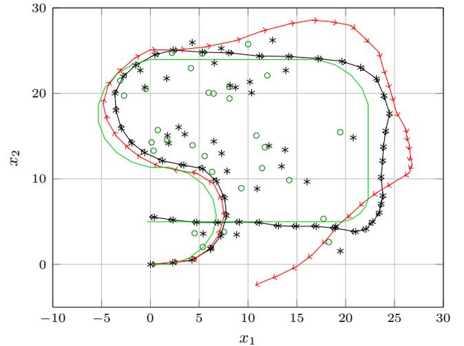
(c) Result with biased range measurements that are treated by the proposed method.
