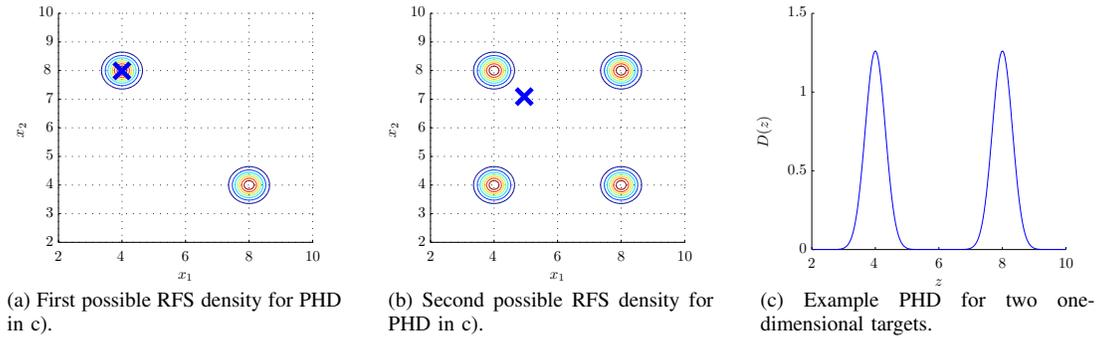
Fig. 2: Example 2: A PHD for two one-dimensional targets and two possible RFS densities. The MMOSPA estimates for the RFS densities (blue crosses) are significantly different.
