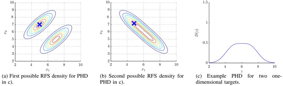
Fig. 1: Example 1: A PHD for two one-dimensional targets and two possible RFS densities. The MMOSPA estimates for the RFS densities (blue crosses) do not coincide.
